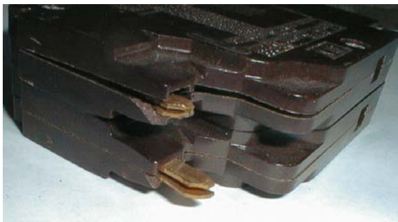
Figure 8 – Damaged “E” type breaker
